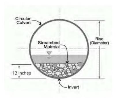
In all other counties: Culverts greater than 48 inches in diameter will be buried at least one foot below the bed of the stream. Culverts 48 inches in diameter or less shall be buried or placed on the stream bed as practicable and appropriate to maintain aquatic passage, and every effort shall be made to maintain the existing channel slope. The bottom of the culvert must be placed at a depth below the natural stream bottom to provide for passage during drought or low flow conditions.
